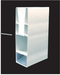
**BOTTOM RAIL:** The foundation of all of our PVC sections is our patented 2" x 6" heavy duty bottom rail with an internal steel support. This rail also features a ridge design for interlocking ability. The increased structural strength of this rail reduces sagging, premature failure, and damage from wind.
